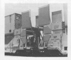
(Above) DTTX 63107 and 63112 showing the new style "streamliner" bulkheads on Southern Pacific's Gunderson built stack container cars. Ed Flaugher photo
