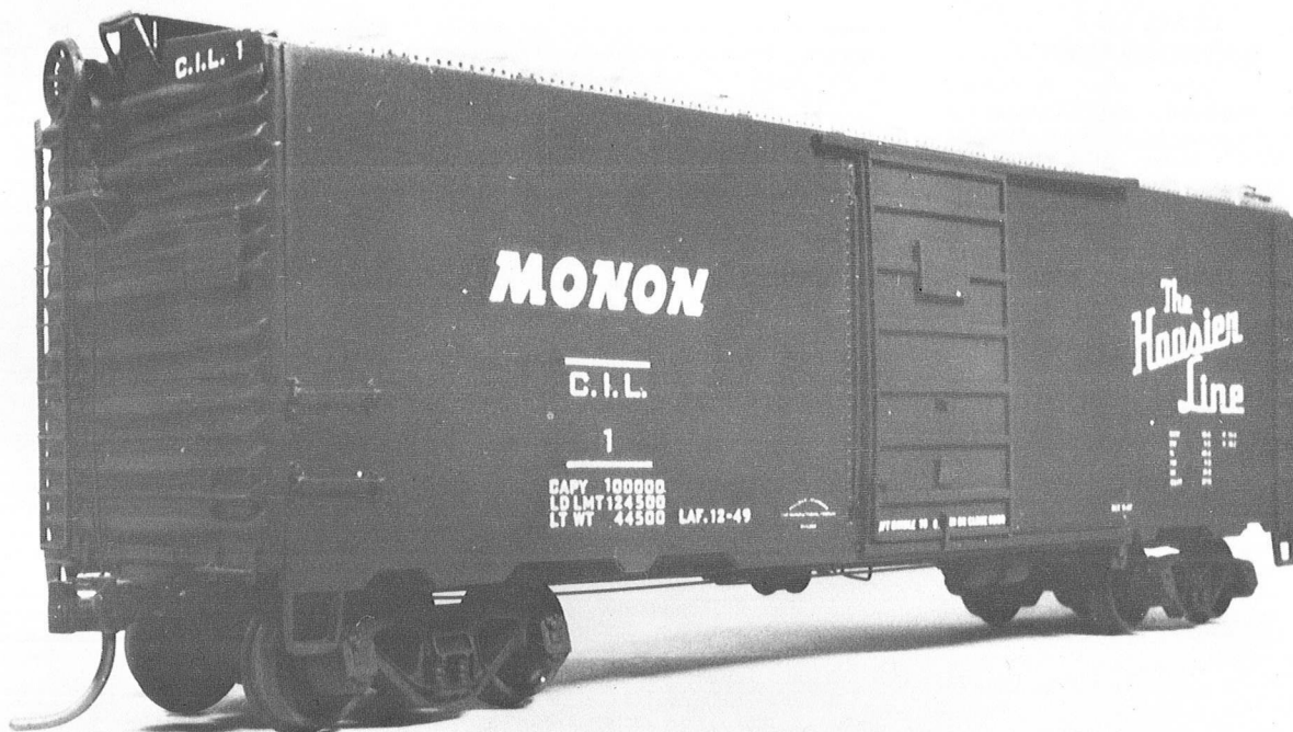
Model of Monon box car N°1 using an Athearn 40' box car body with reworked sides to simulate welded construction, ends built up from Athearn 40' reefer ends and scratch built doors. The prototype was built by Pullman-Standard in 1947. Pictures of Monon N° 1, and sometimes of cars with their number retouched to "1" by an ambitious PR department, were used to advertise the innovative management the Monon had in the late 1940's and 1950's. In the late 1960's Monon N° 1 was renumbered 10053. Staffan Ehnbon.
