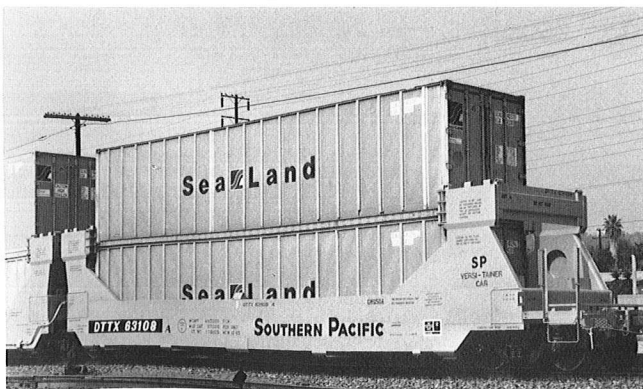
DTTX 63108, basically a standard Gunderson car. Shown is the "A" unit. (Ed Flaucher photo)
