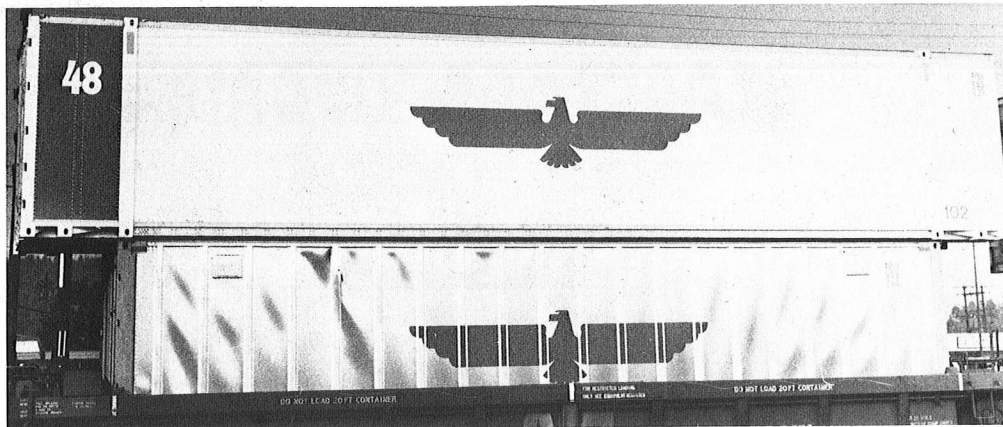
(ABOVE) APLU 480035, the new 48' long by 102" wide containers. Note how this one sits on the lower 40' container. Colors are white container with red and front band, white 48 on side. All other lettering is blue including numbers, data, etc. (Ed Flaughter photo)
