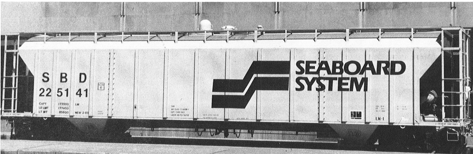
Seaboard 225141, built by Thrall's United American Division in 2-85 is a combination covered hopper and tank car for molten sulphur loading. (Richard Yaremko photo)
