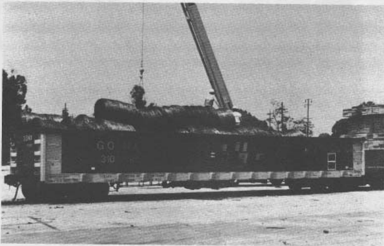
ABOVE: GONX 310999, filled with bundles of steel wire, gets offloaded by a small capacity Grove mobile crane in Ontario, California on the SP. This car, built by Thrall Car is part of Railgon's second largest series of gondolas in their fleet. (D.G. Casdorff)
