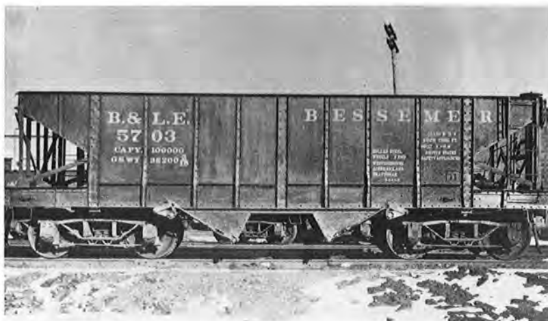
Figure 2. Type II - Production version of the Type I, one of 400 built in 1897. Shown as rebuilt in 1915; 50-ton capacity, 28 foot inside. A.J. Colantuono.
