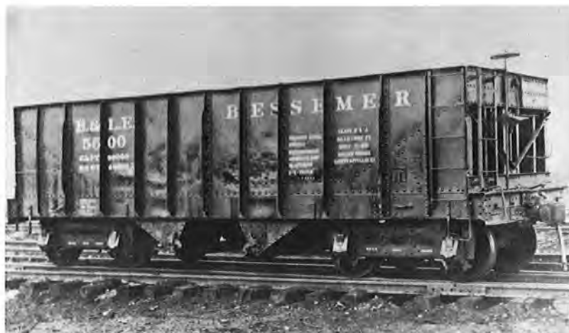
Figure 1. Type I - One of two experimental cars built in 1896, photographed on its 20th anniversary. A.J. Colantuono.
