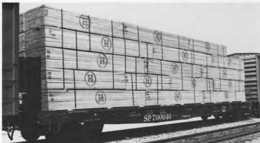
(ABOVE) Southern Pacific 700040, part of a series of newly acquired rebuilt general-service flats for lumber service. Built in 1966 and rebuilt in May 1986 by Gunderson, the car is a General Steel Industries design. SP has assigned a new class to this series of cars; F-70-92-G. David G. Casdorff photo
